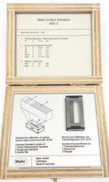
Mahr MSS-3 certified surface and step standard
