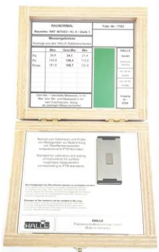
Halle – super fine certified surface roughness standard
